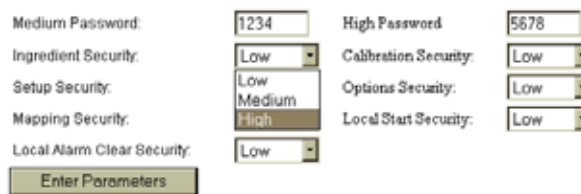
FIG. 334: CONFIGURATION - SECURITY/ PARAMETERS SET FOR SECURITY LEVELS
