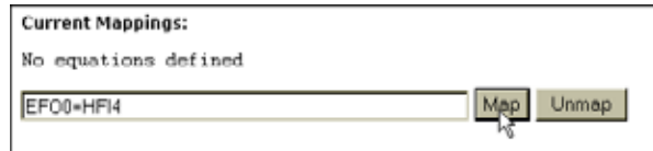
FIG. 269: GROSS WEIGHT-CHANNEL 1 ASSIGNED TO HARDY CONTROL-LINK FLOAT OUT
