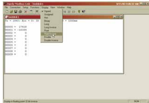
FIG. 174: HARDY MODBUS-LINK DISPLAY/ SELECTING DISPLAY/FLOAT INVERSE
