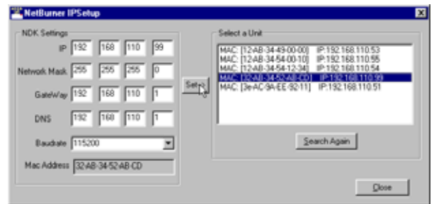
FIG. 34: IP SETUP MENU
