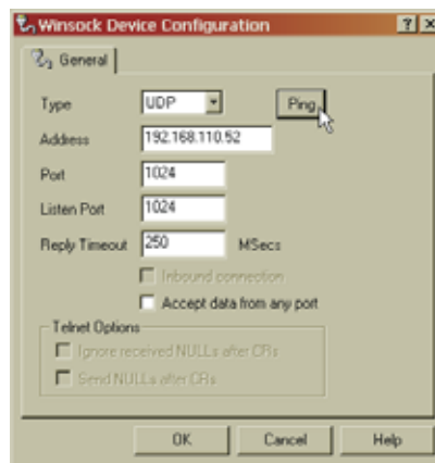
FIG. 188: WINSOCK CONFIGURATION/ENTERING HI 3000 SETUP PARAMETERS
