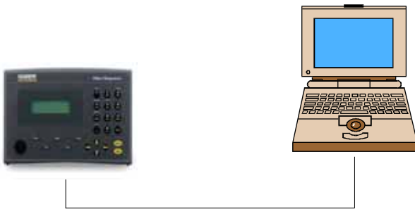
FIG. 90: SIMPLE HARDY CONTROL-LINK NETWORK
