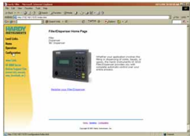
FIG. 69: HI 3000 HOME PAGE/SELECTING CONFIGURATION
